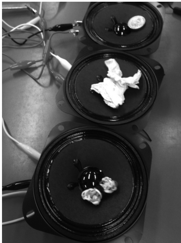
Figure 1. Open experimentation with the Victorian Synthesizer, a musical instrument made from hacked loudspeakers based on electro-mechanical principles.
